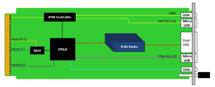
Figure 3: AMC080 Functional Block Diagram
