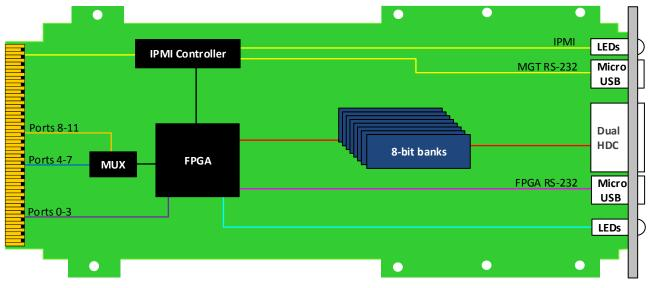
Figure 4: AMC080C Functional Block Diagram
