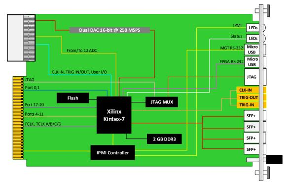
Figure 2: AMC523 Functional Block Diagram
