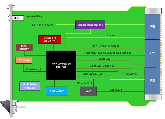
Figure 4: VPX705 Functional Block Diagram
