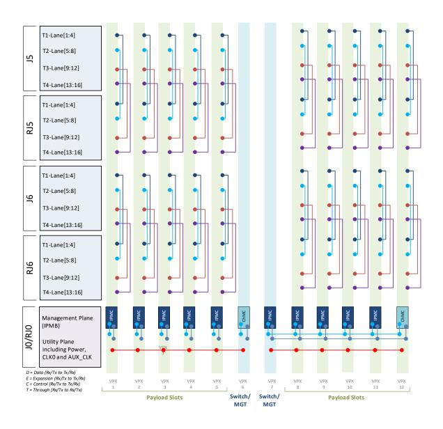
Figure 4: VTX866 Backplane Connections J5-J6 and J0
