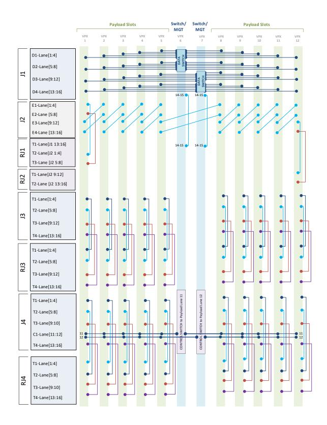
Figure 3: VTX866 Backplane Connections J1-J4
