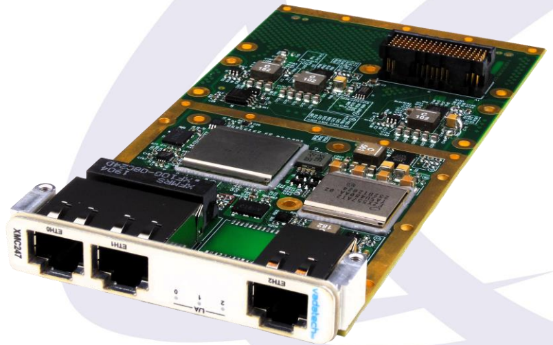
Figure E: XMC247 A=2 without Heatsink
